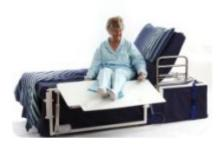
Powered leg lifters are powered devices that attach to the bed frame and require the user to sit on the edge of the bed with their feet on the floor and in front of the device. They work on the principle of a platform that raises through an arc of 90 degrees, lifting the legs of the user to a position just beyond the horizontal, level with the mattress. From this position, the user can slide their legs off the platform and onto the bed.
